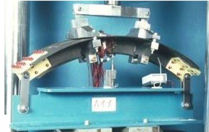
**Air Frame rupture test**
