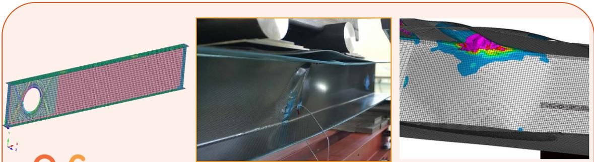
Damage analysis accounting for mechanical properties resulting from manufacturing
