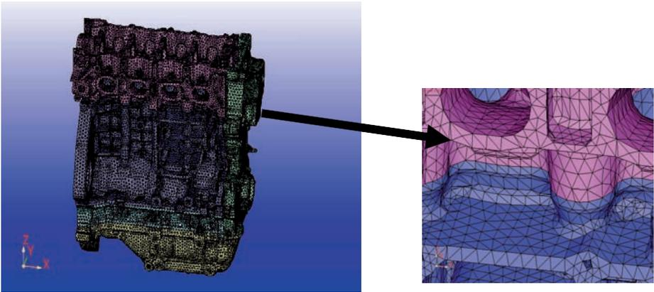
*Fig. 4.5.4.1: Example of automatic assembly meshing
