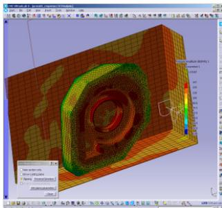
Save potentials to see how well the waves are actually attenuated in PML layer
