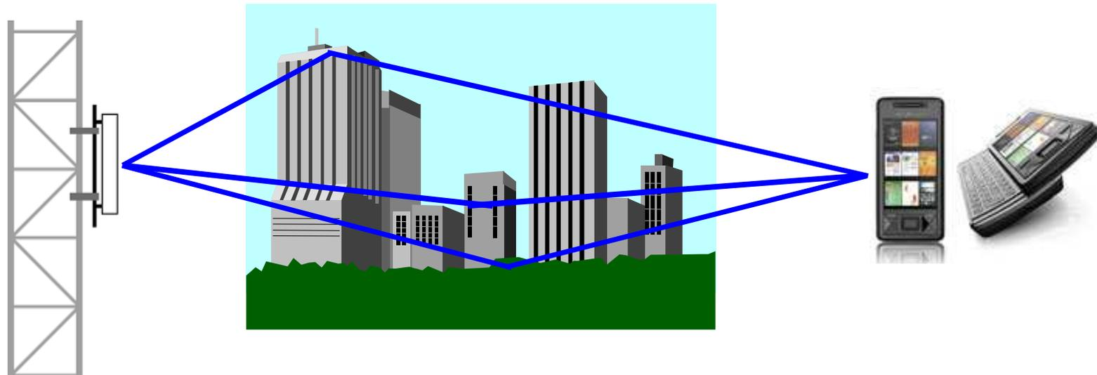
Base Station Parallel data streams to increase capacity Handheld
