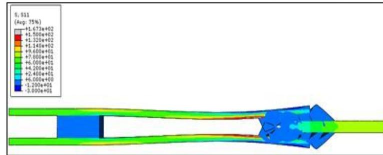
Axial Stress with Displacements  $\times 10$
