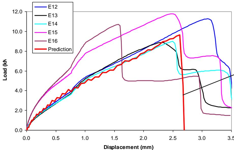
Analysis with failure prediction and failure criteria: effective plastic strain 56.5%.
