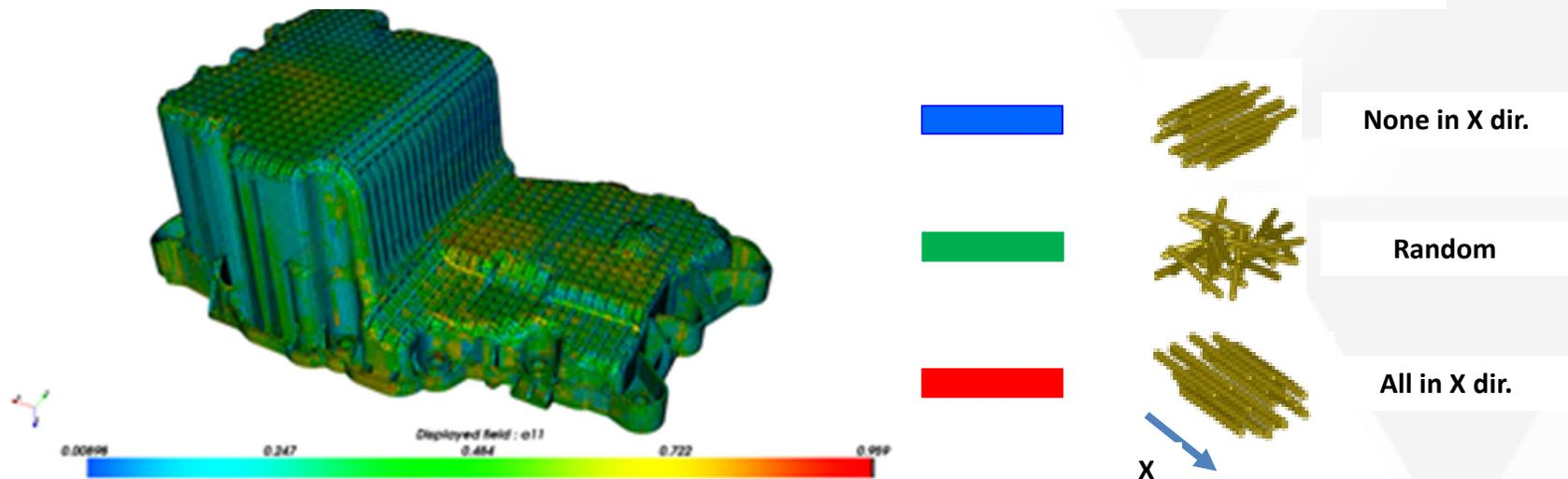
Note : complete tensor includes 6 coefficients : a11, a22, a33, a12, a23, a13
