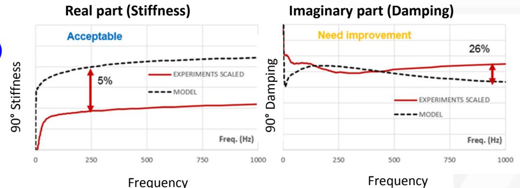
Experimental scaled curves = post processed curves from measurements on 3 samples
