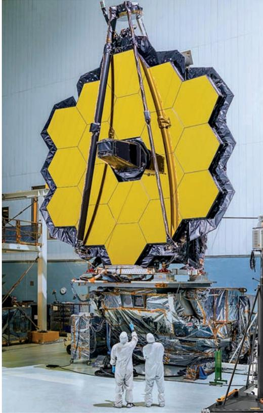
**The primary mirror of NASA’s James Webb Space Telescope, consisting of 18 hexagonal mirrors, looks like a giant puzzle piece standing in the massive cleanroom of NASA’s Goddard Space Flight Center in Greenbelt, Maryland.**
