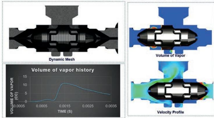
**Subsea valve cavitation study**
