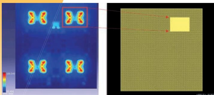
**Using ML to automate the detection of chip hot spots by applying fine meshes where they are needed.**
