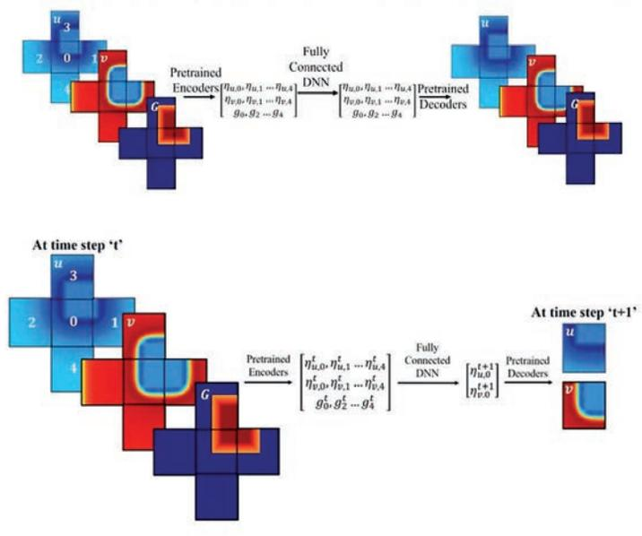
**Steady-state (top) and transient (bottom) flow solvers for the Navier-Stokes equations focusing on small regions at a time.**
