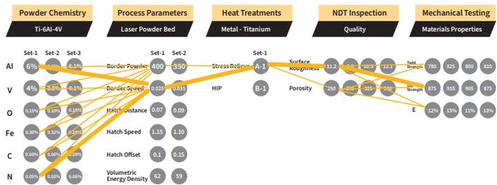
Using machine learning to identify the causal links between AM data
