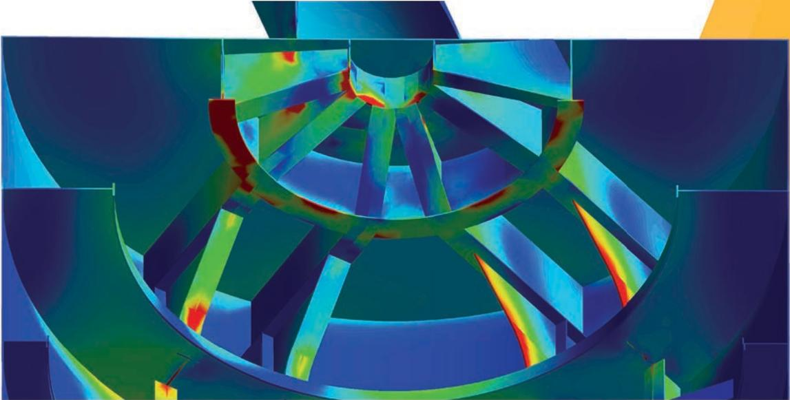
**Interior view of the starboard column, showing the internal reinforcements under the main mast connection**
