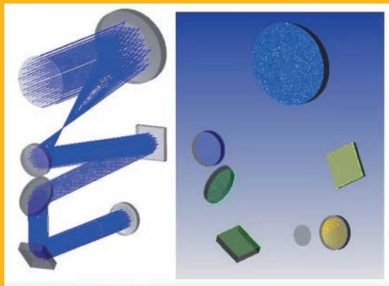
Using the Ansys Zemax OpticStudio STAR software to add deformations (generated by finite element analysis) to the optical model of a mirror system
