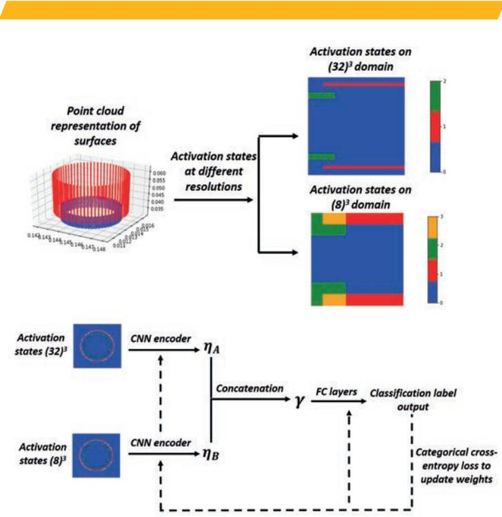
**The ActivationNet algorithm uses the spatial location and density of points in a cloud or mesh to generate activation states (top). Depending on the problem at hand, these activation states reflect the geometric model at a range of resolutions. The collected activation states, which represent contact-surface interactions, are handed off to neural networks for assessment (bottom).**
