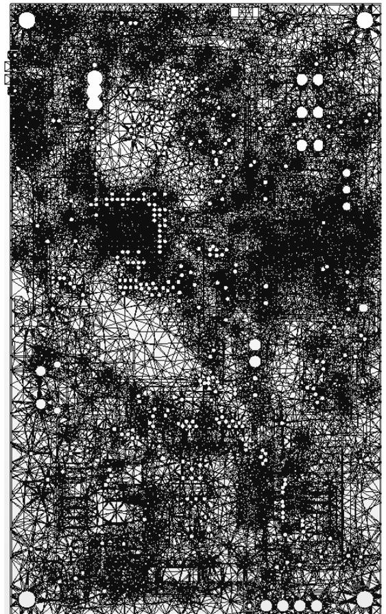
Figure 9. Final mesh of the PCB
