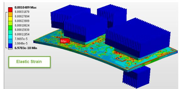
Figure 23. Elastic strain
