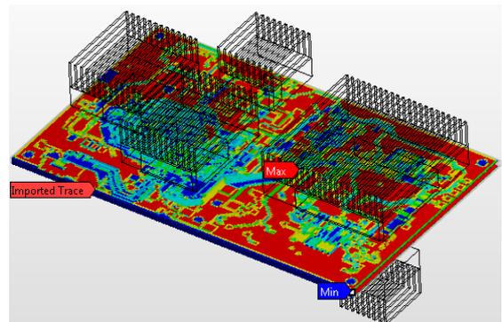
Figure 19. Imported layer metal with heat sinks
