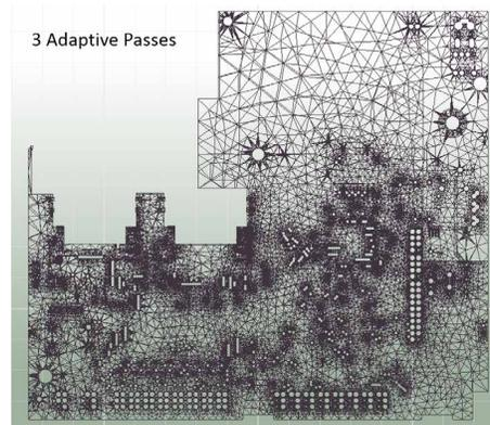
Figure 7b. Adaptive mesh after three passes
