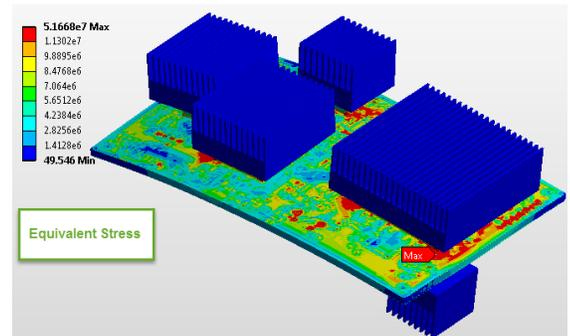
Figure 22. Thermal-induced stress
