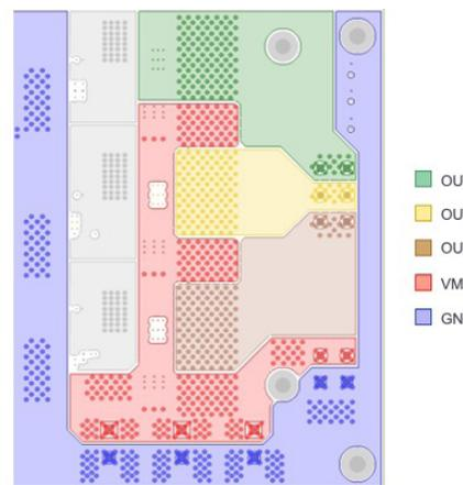
Figure 4: EVALSTDRIVE101 first inner-layer PCB
