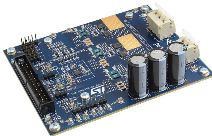
Figure 1: EVALSTDRIVE101 demonstration board
