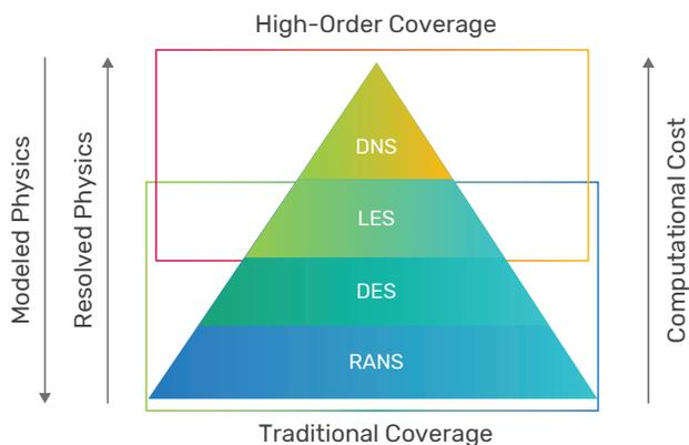
Figure 4: Expanding Fidelity CFD turbulence modeling from traditional to high-order coverage
