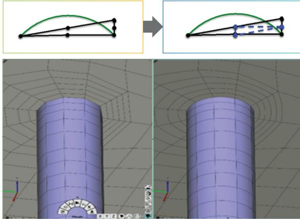
Figure 3: Interpolating linear mesh to mesh for reduced cell count, reduced memory requirements, and unprecedented accuracy
