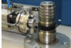
Instrumented Chip & Cut Analyzer
