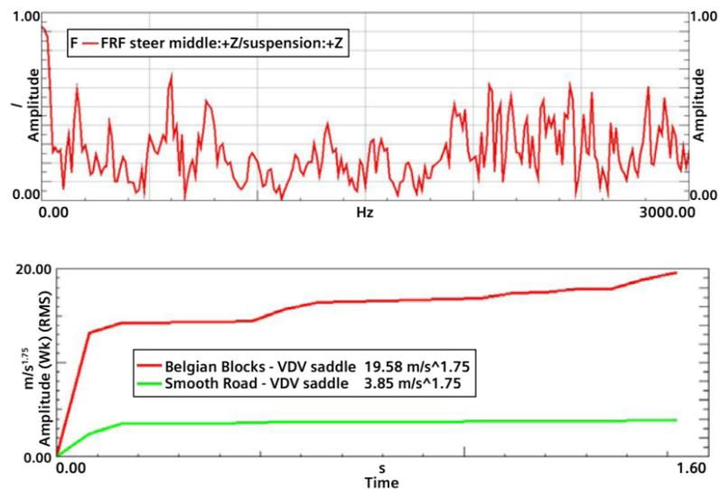
the motor itself, I had to understand how much noise was generated by the road surface. I cleaned up the data collected from riding over both cobbled and smooth paths using sound quality metrics such as Articulation Index, Prominence Ratio, and Time Varying Loudness as well as adding traditional SPL and Spectrum analysis.
