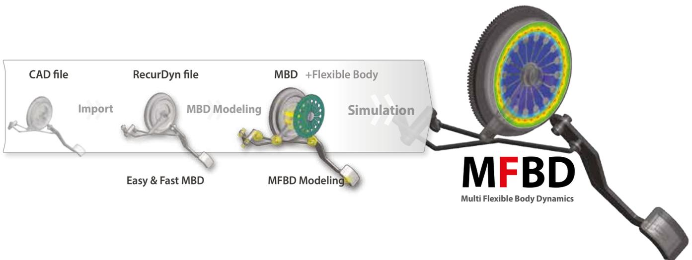
The MBD analysis results include the position, velocity and acceleration of each body and the reaction forces or frictional forces at each constraint (joints, etc.) as well as forces at each contact. With these outputs, you can view and understand the dynamic behavior of the system. Flexible bodies output stress and strain.
