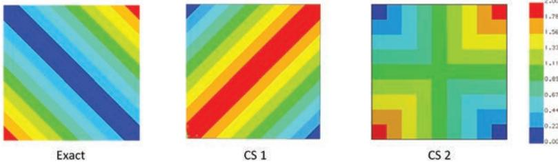
**Figure 9: Contour plots of von Mises stress for the challenge problem**
