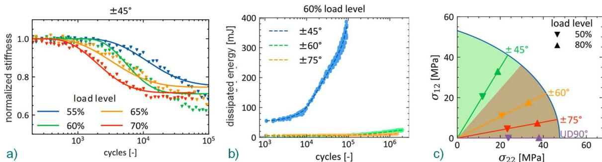
Fig. 2 (adapted from [9]): Change in axial stiffness of a ±45° angle-ply laminate at various load levels normalized to its initial stiffness – model (solid lines) vs. experiments (data points) (a); dissipated energy obtained from hysteresis evaluation of experimental data (b); ply stress states for the laminates investigated plotted for in-plane shear vs transverse tension stress (c).
