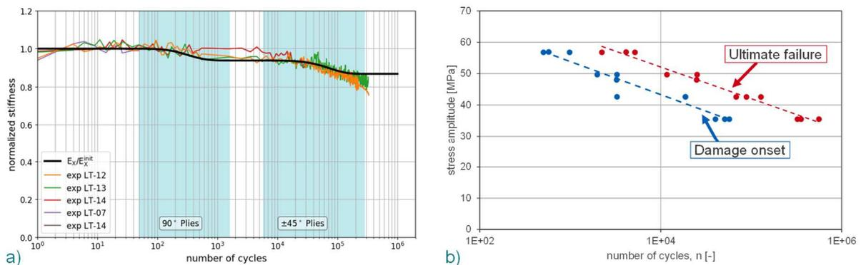
Fig. 3: Change in axial stiffness of a multi-axial laminate with  $[0/45/90/-45/0]_s$  layup normalized to its initial stiffness – model vs. experiments (a); SN-curves for damage onset and ultimate specimen failure for a  $\pm 45^\circ$  specimen (b).
