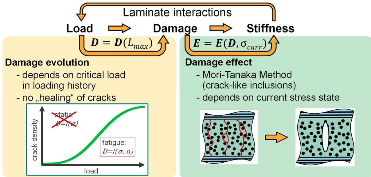
Fig. 1: Two-step modeling concept with a distinct separation of damage evolution and damage effect.
